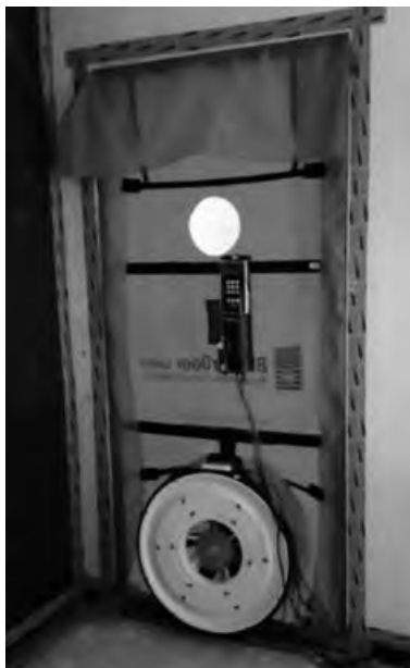
Figura 4: Ensayo Blower Door.
